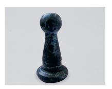
Part finished with **Zinc Nickel PLUS Black** after 4,800 hours in neutral salt spray testing shows no sign of red rust.
